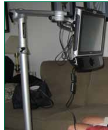
EyeGaze device on a rolling mount allows for communication access in a variety of locations around the home.
